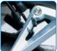
Bungee hooks shown attached correctly to a solid anchor point
